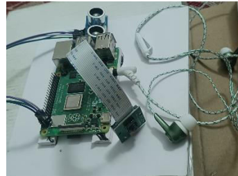
FIG.3.EXPERIMENTAL SETUP OF THE OBJECT RECOGNITION AND DISTANCE MEASUREMENT DEVICE
